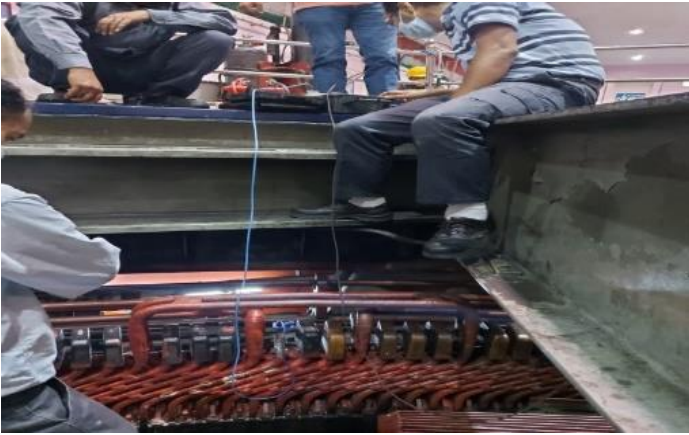
Figure 3. Testing of Stator Sections
